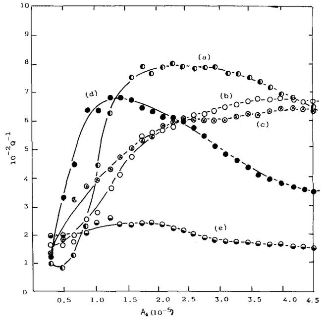
Fig. 6. Internal friction peaks (versus strain amplitude) of Al bicrystal with misorientation angle 60° measured at several temperatures within the temperature range of the internal friction peak shown in Fig. 5: (a) 55, (b) 105, (c) 128, (d) 188, (e) 247 °C.
