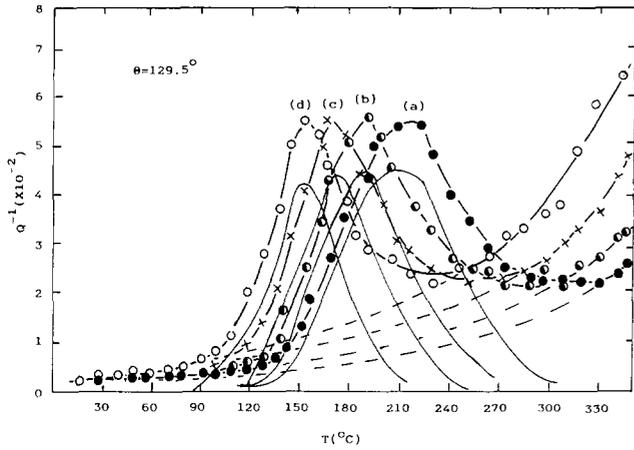
Fig. 3. Internal friction peaks of Al bicrystal with misorientation angle 129.5°, measured with frequencies: (a) 1.5, (b) 0.483, (c) 0.155, (d) 0.05 Hz.  $f=1$  Hz,  $A_\epsilon=1 \times 10^{-5}$ .
