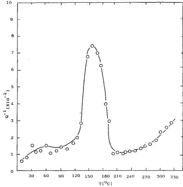
Fig. 5. Internal friction peak (versus temperature) of Al bicrystal with misorientation angle 60°.  $f=1$  Hz,  $A_\epsilon=1 \times 10^{-5}$ .
