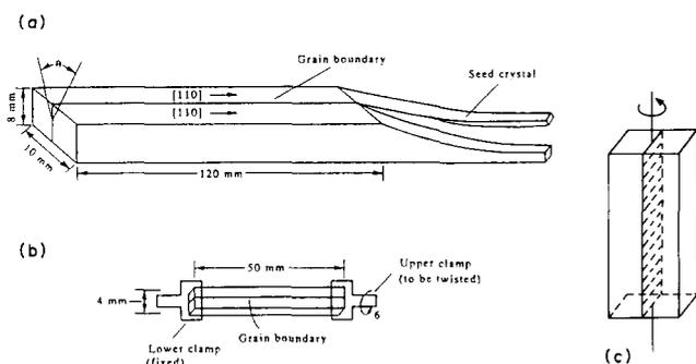
Fig. 1. (a) The as-received aluminium bicrystal; (b) specimen used in internal friction measurement; (c) torsional stress applied to the specimen.
