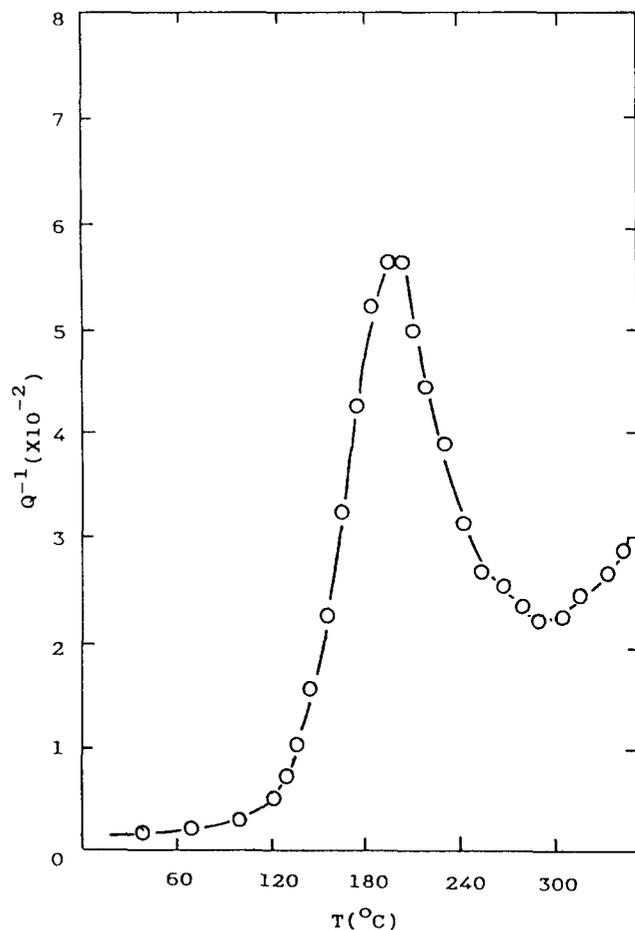
Fig. 2. Internal friction peak (versus temperature) of Al bicrystal with misorientation angle 129.5°.  $f = 1 \text{ Hz}$ ,  $A_e = 1 \times 10^{-5}$ .
